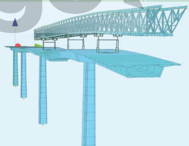
at the final stage, different result envelopes are required. The specific construction stage manager separates and combines the different stage effects into action envelopes, providing maximum and minimum forces, displacements and stresses for quick result access for both the bridge structure and the gantry. All the special tasks such as the support uplift are, naturally, taken into account as part of the staged analysis. Sofistik has been used here for a couple of individual scenarios such as a
